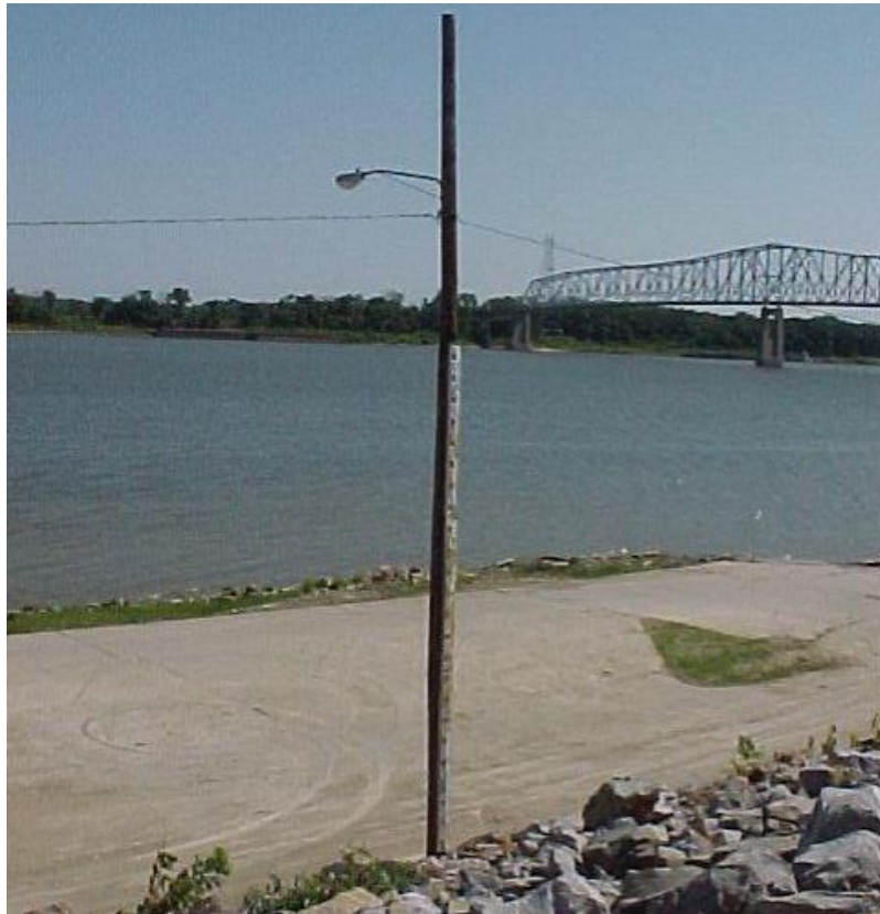
Figure 4.5: Staff gauge on a light pole
